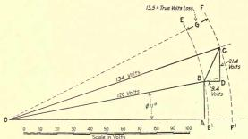
Fig. 114.—Solution with 300,000-cir. mil conductors.
